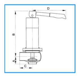
Designed to meet the changing needs of the process industry, the new Series 3 Pressure Relief valve uses elements of the DPL single and double seat valves to produce a full bore, self draining device ranging in size from 1-4".
